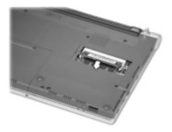
Note The system switches are also located in the memory module bay. Therefore, if you need to set any system switches, you might want to do so while the system is already disassembled. The system switches are defined in Chapter 3.
